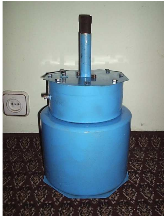
Fig. 5. The photograph of the Faraday's cage.
