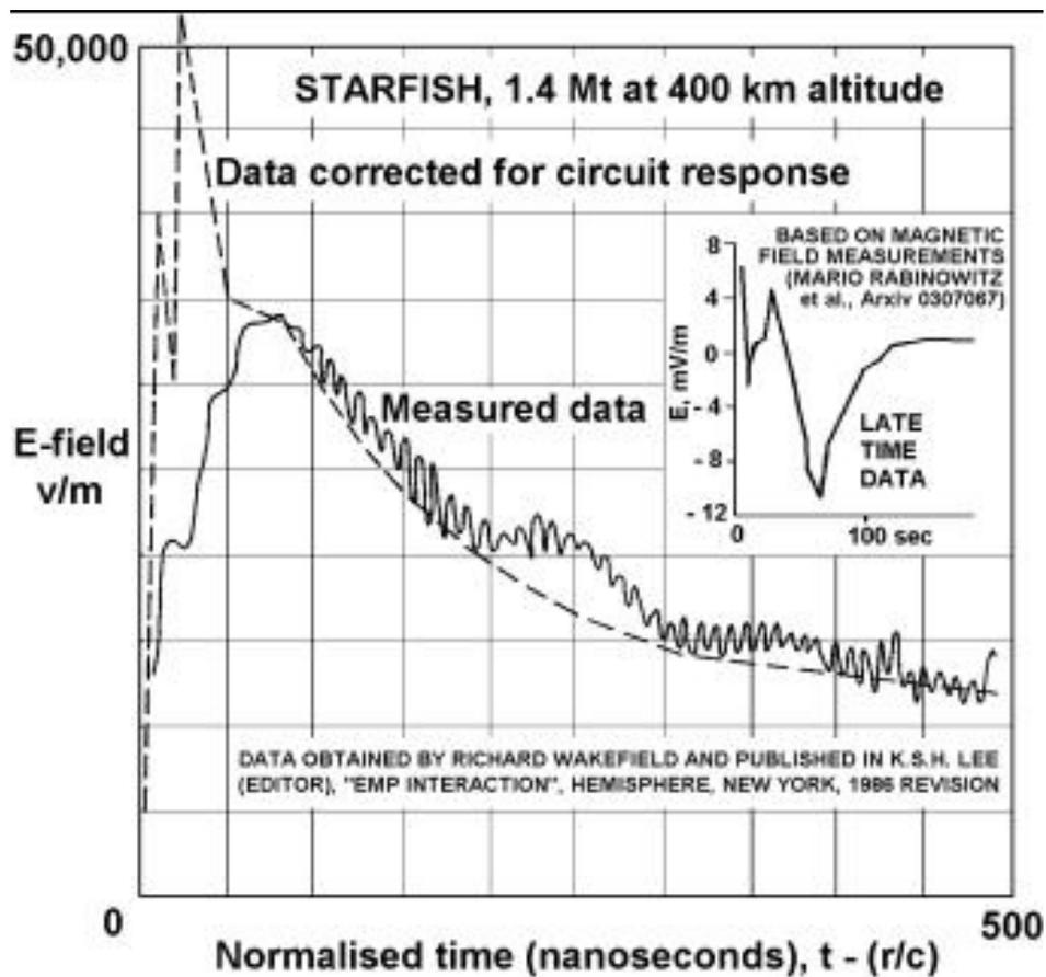
Fig. 13. Experimental dependence of amplitude EMP on the time, obtained with the tests according to the program *Starfish*.
