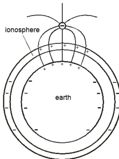
Fig. 16. Negative charge above the earth's surface with the presence of the ionosphere.
