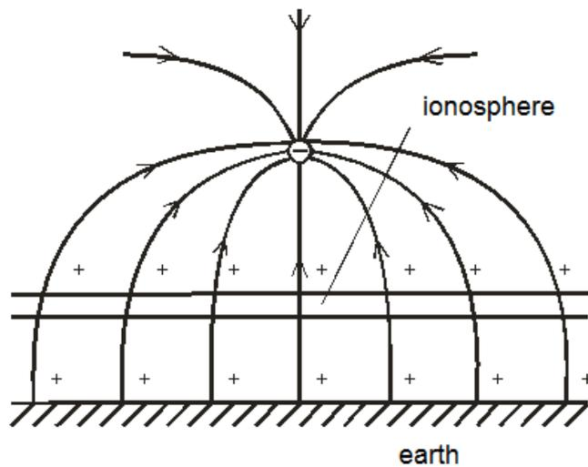
Fig. 15. Negative charge above the earth's surface with the presence of the ionosphere.
