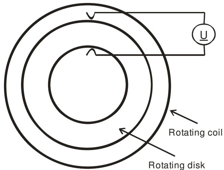
Fig. 8. Schematic of unipolar generator with the revolving turn with the current and the revolving conducting ring.
