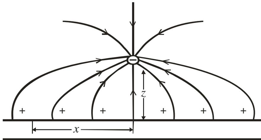
Fig. 14. Negative charge above the limitless conducting plane.
