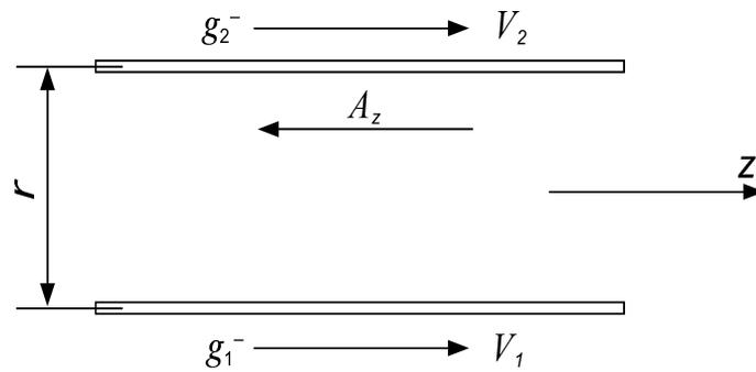
Fig. 3 Schematic of power interaction of the current carrying wires of two-wire circuit on the basis of the existing model.
