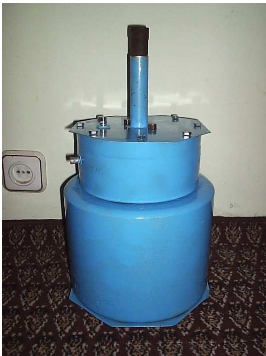
Fig. 21. The photograph of the Faraday cage.
