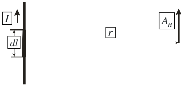
Fig. 2: The formation of vector potential by the element of the conductor dl , along which flows the current I
